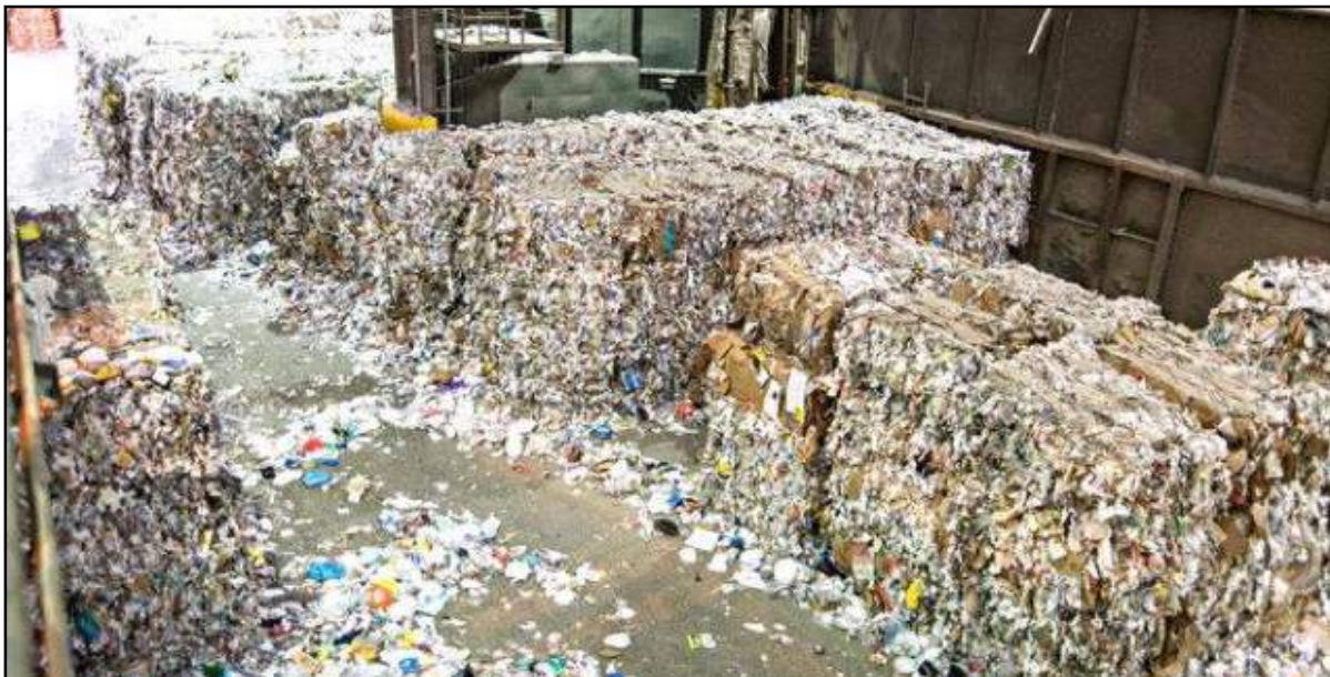
Figure 36: Baled waste paper ready for distribution to recycled paper manufacturing facilities (Source: InSitu)
