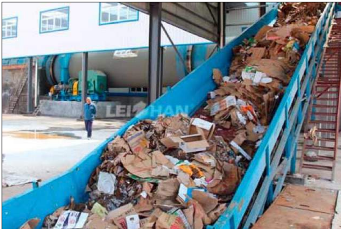
Figure 37: Higher quality cardboard waste paper being input to the paper production process (Source: InSitu)
