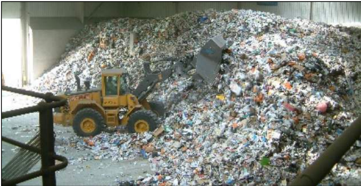
Figure 35: Loose, sorted waste paper being prepared for baling (Source: InSitu)
